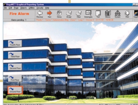
Level 1 page Showing building floor level in alarm
